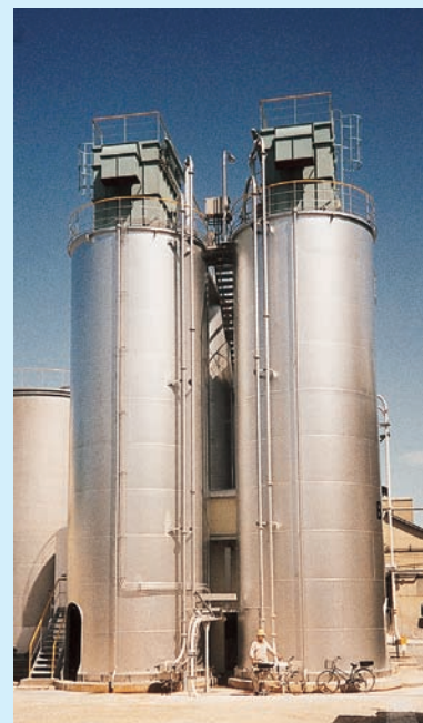
100TON/Batchx4 Air blend silo for special cement
