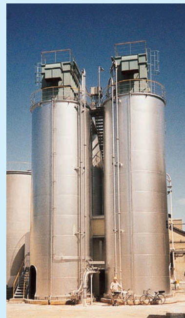
100TON/Batchx4 Air blend silo for special cement
